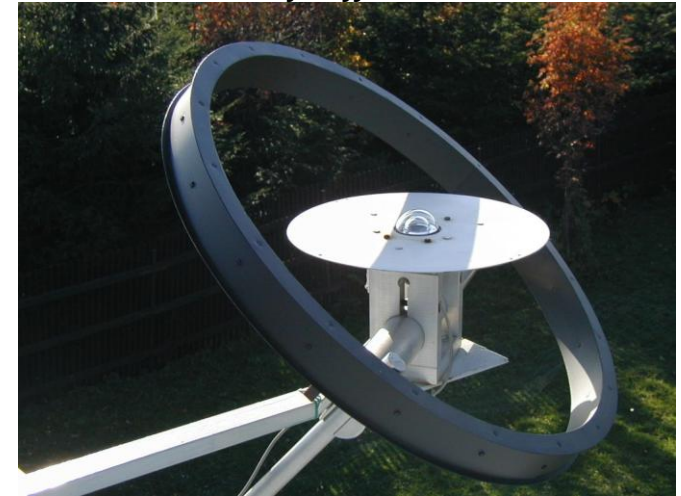
Solarimeter Kipp-Zonnen – measurement of diffuse radiation
